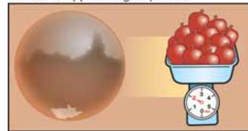
Figure 2.7: Fifteen apples on Earth weigh 5 pounds. The same 15 apples weigh 2 pounds on Mars! This is because the force of gravity is less on Mars.
