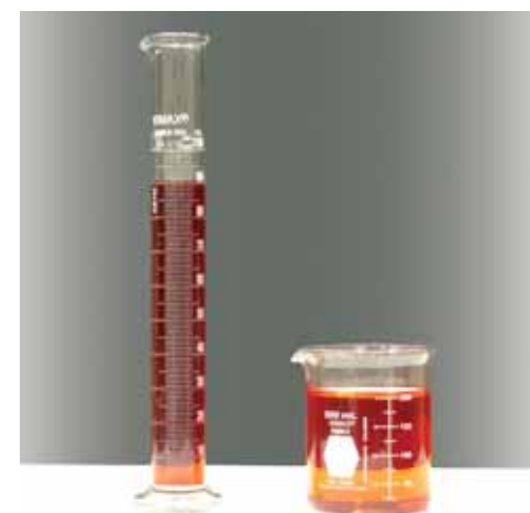
Figure 2.6: A beaker and a graduated cylinder are used to measure small volumes.
