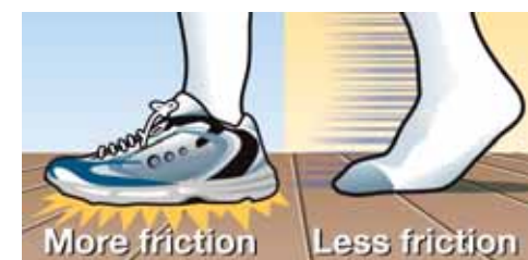
Figure 9.2: There is more friction between a sneaker and a gym floor than between a sock and the gym floor.
